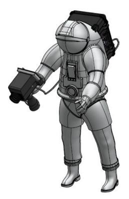
Design of a handheld multi-analytical spectrometer for use by astronauts during Lunar exploration missions. Credit: University of Leicester and ESA.
