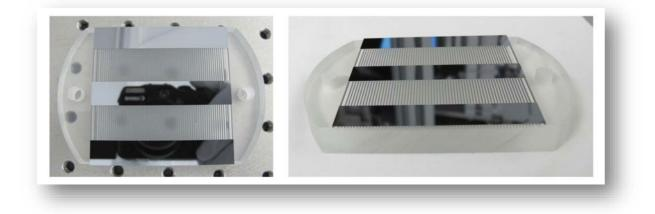
Prototype "slatted mirrors" have been machined from silicon wafers and are approaching the performance needed to create an interferometer. Credit: Willingale et al. Proceedings of the SPIE, Volume 8861, id. 88611S 6 pp. (2013).
