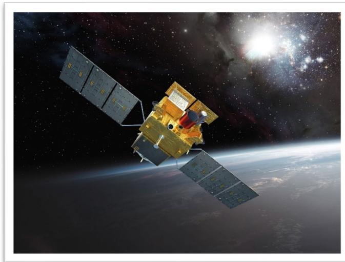
The SVOM satellite. The Space Variable Objects Monitor (SVOM) satellite. SVOM carries four instruments providing coverage from optical to MeV energies. The project also has several ground-based telescopes observing in the optical and IR. Credit: CNES
