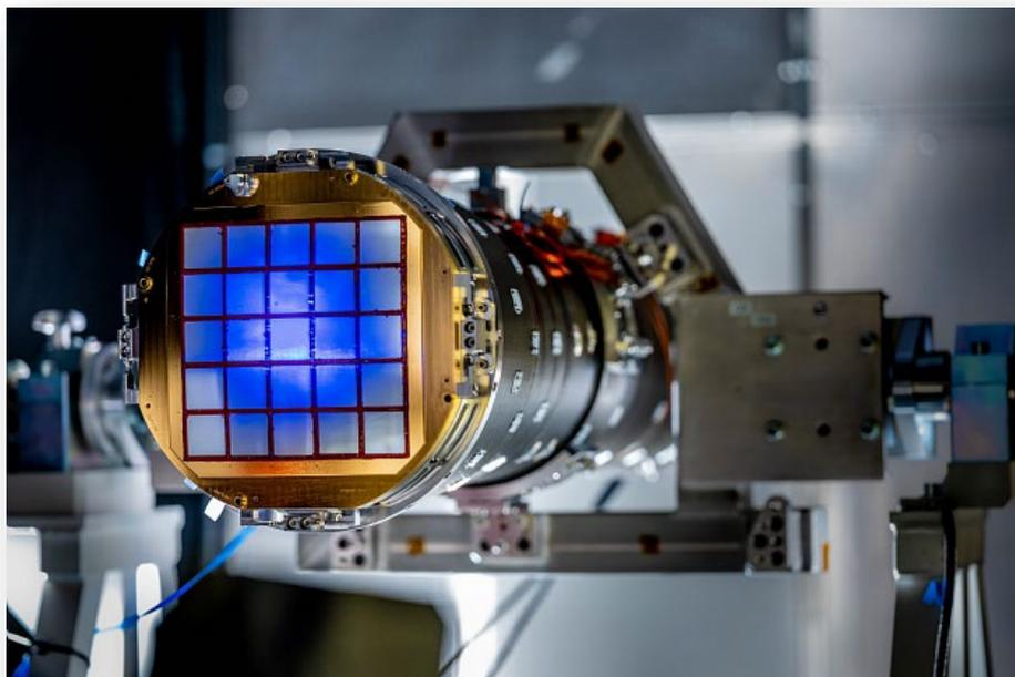
The SVOM MXT flight instrument using a lobster eye optic designed and built at the University of Leicester. (© CNES/DE PRADA Thierry, 2021)
