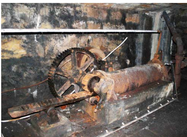
Figure 3. Alnwick Castle, Northumberland: hydraulic machinery for dumb waiter, c. 1860s. The castle had many other early examples of hydraulic lifts
