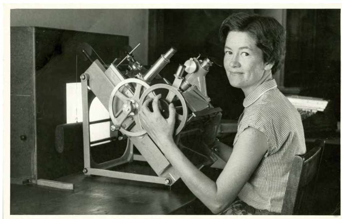
Figure 3:4 Winsome Bellamy using the Hilger Measuring Machine, 1960s. Reproduced courtesy Winsome Bellamy, Collection: Sydney Observatory.
